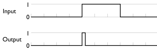
Figure 7.9: Rising Edge Contact
