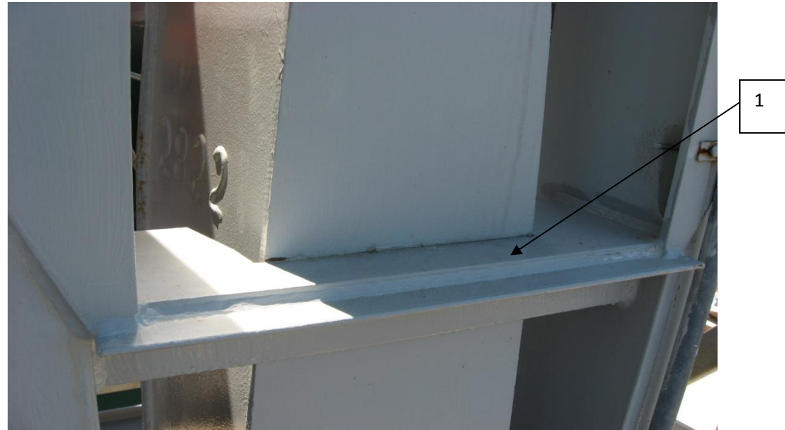
Photo of a davit up tight against the upper davit stop (1) . In this position the davit travel inward is stopped.
