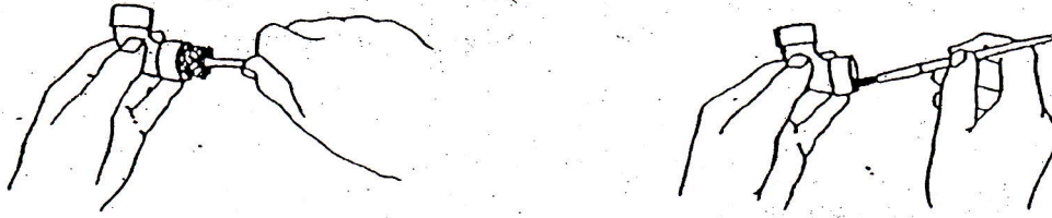
Cleaning the fitting and applying the flux.
