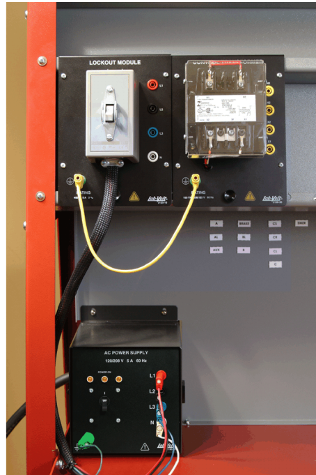
Figure D-3. Lockout Module connected to the AC Power Supply module.
