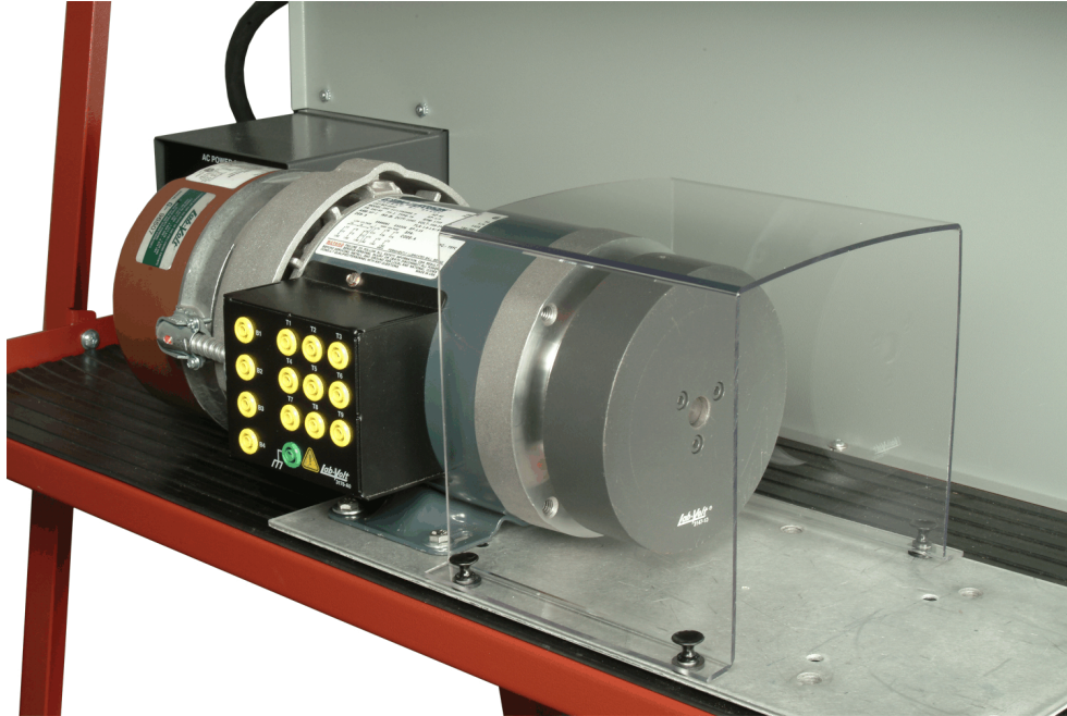
Figure E-4. Installation of the Safety Guard.
