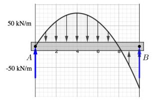
1. Determine the total downward force due to the distributed load. Consider the load to be made of an infinite number of infinitesimal weights dW = w(x) dx.
