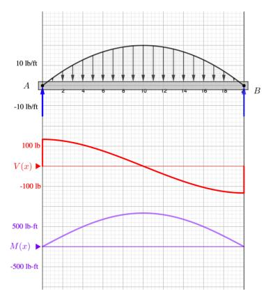
The equivalent downward force of the distributed load is the "area" under the loading curve.
