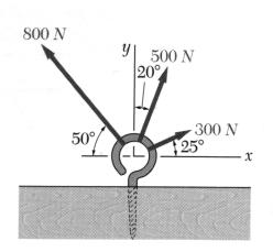
**Example 3** A hoist trolley is subjected to the three forces shown.
