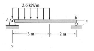
2. Replace the distributed loading with an an equivalent resultant force and specify its location on the beam measured from *A*. Determine the reactions at *B* and *C*.
