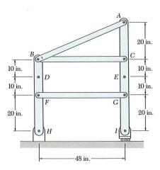
Determine the components of the reactions at D and E if the frame is loaded as shown.
