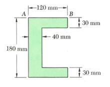
Determine the moment of inertia and radius of gyration of the shape with respect to the *x*-axis.
