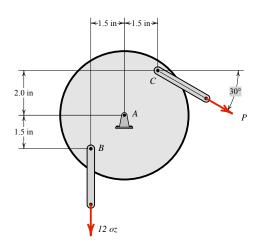
2. Using the principle of two- and three- force bodies, determine the forces acting on the cylinder at points A and B.
