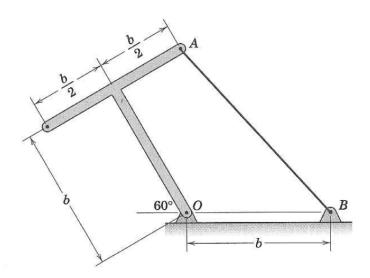
2. Determine the moments of the tension T about point P and point O.
