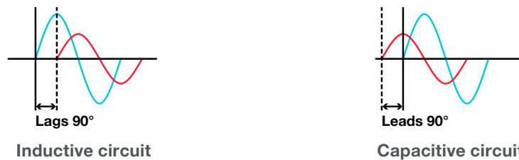
Figure 14 - Phase offset between voltage and current with a purely inductive or capacitive load
