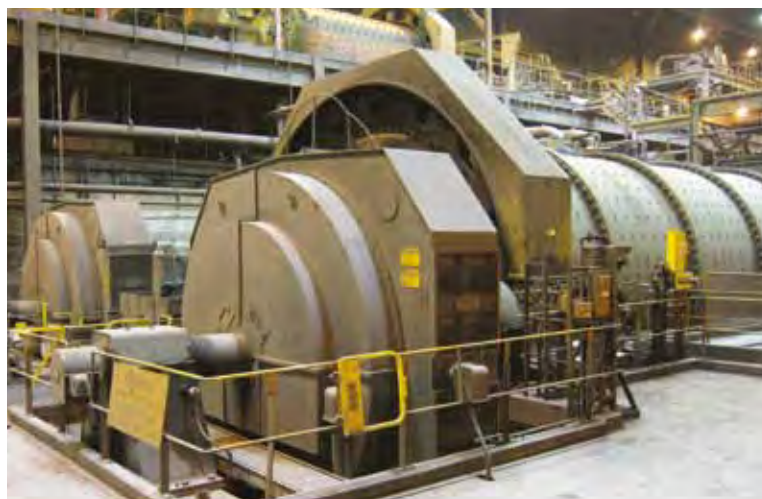
Synchronous motors 3000 HP at 164 RPM with DPG enclosures driving a dual pinion ball mill at an iron ore mine.
