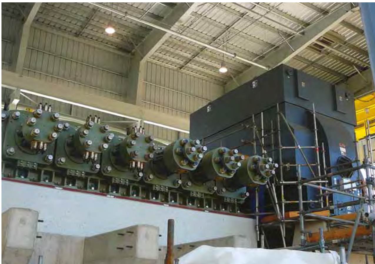
Synchronous motor 24800 HP at 225 RPM with TEWAC enclosure driving a reciprocating compressor at a polyethylene plant.
